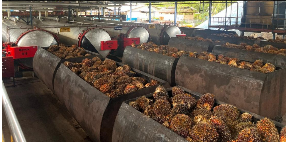
Figure 6. Horizontal Cooking at Mill #1
