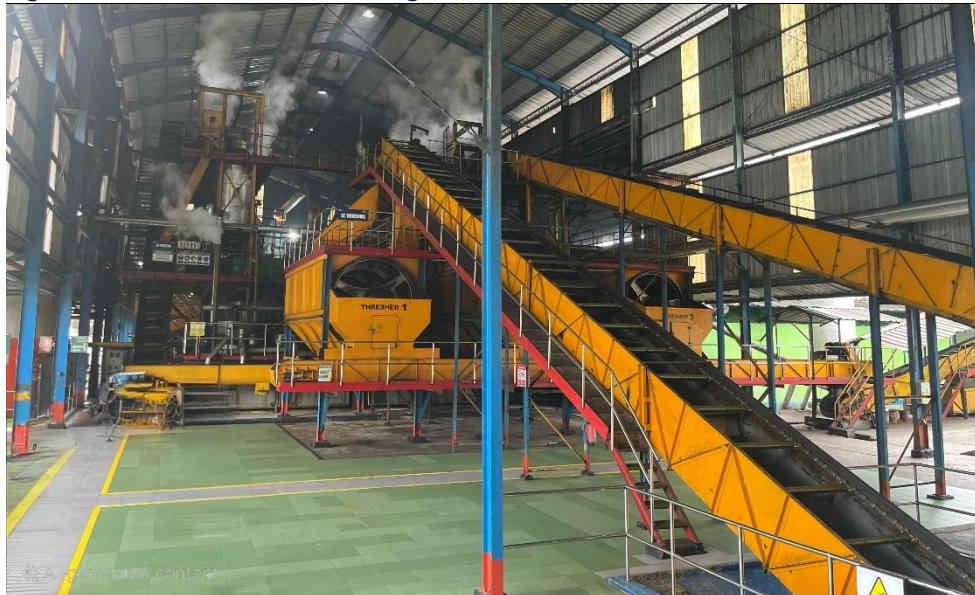
Figure 7. Mill #1 Horizontal Cooking Method
