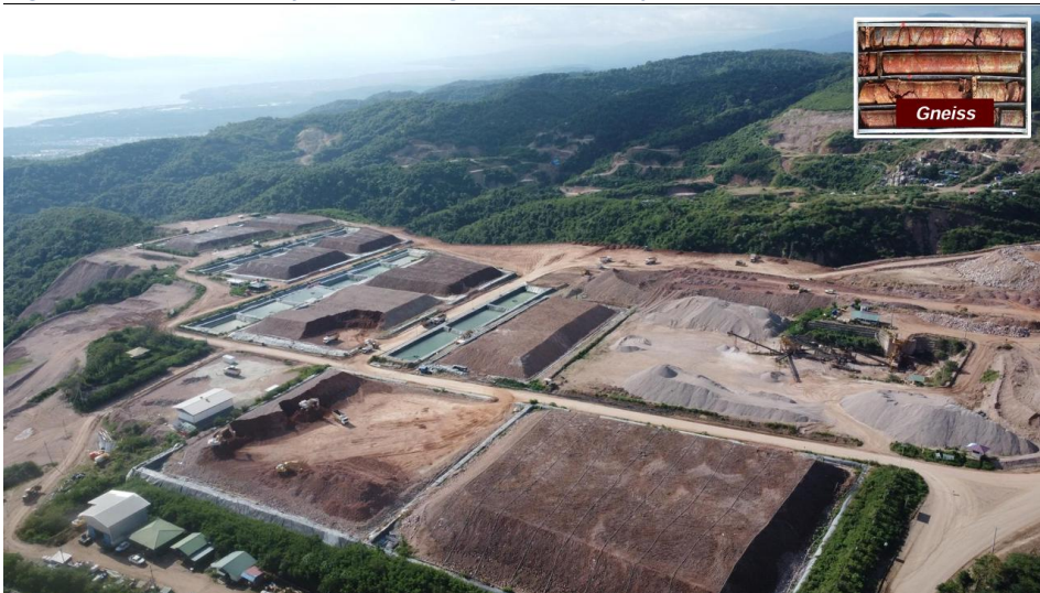
Figure 4. Block-1 Poboya Processing Plant #3 (Heap Leach Method)
