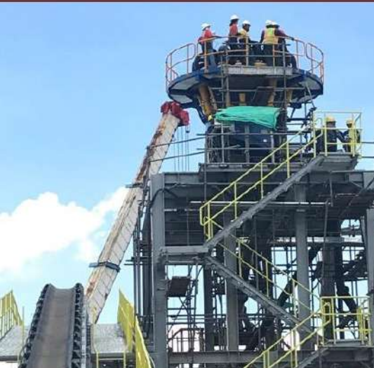
Cyclone to separate the fine ores (-75 um) from the coarse ores (+75 um)
