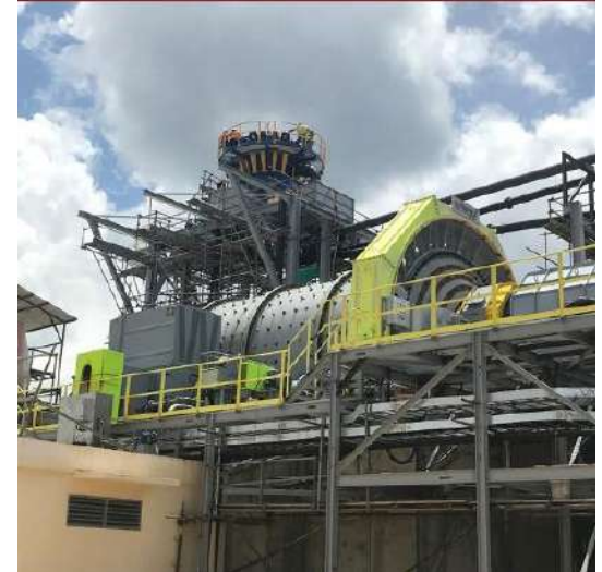
Ball mill to grind the ores from size 12 mm to become -75 um
